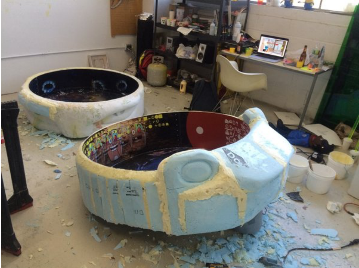
the sculpted foam exteriors being added
